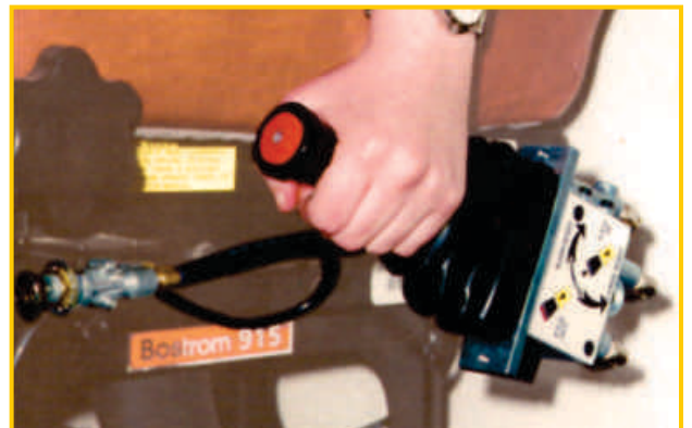
Operating the P.T.O. and Dump.
